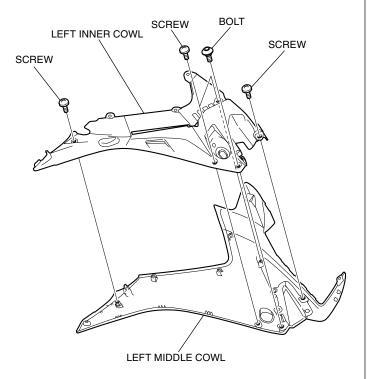
9. Remove the existing left lower headlight cover as shown.
